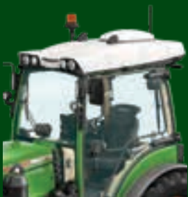
The Fendt Guide receiver is well protected and integrated into the roof design.
